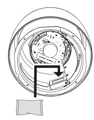
**IMPORTANT!** If the bubble is attached to the dome for up to 30 minutes or more and then detached, the bag must be replaced before the bubble is attached again. An extra bag is supplied. If more are needed, order kit 0352-0207-02.
